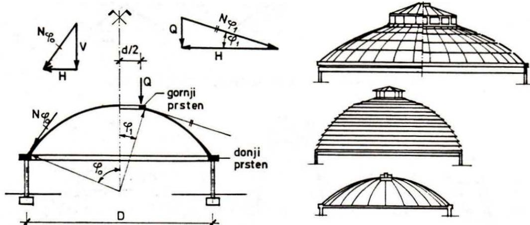
$$D = 10 - 100 \text{ m} \quad d/r > 1/600 \quad d = 5-14 \text{ cm}, \quad \sigma_b < 0,5 \sigma_{b,dop}$$
